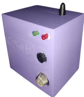
Figure 4. Prototype of gas leakage detector (GD-M5)
