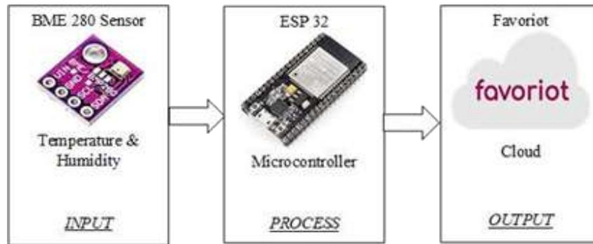
**Figure 1: The block diagram of the mushroom cultivation environment monitor**
