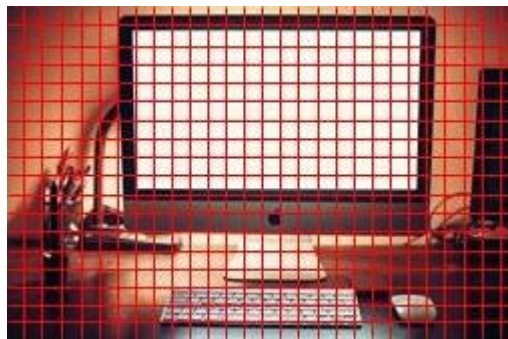
Figure 1. Illustration of an image partitioned into 28 \times 18 small square blocks.
