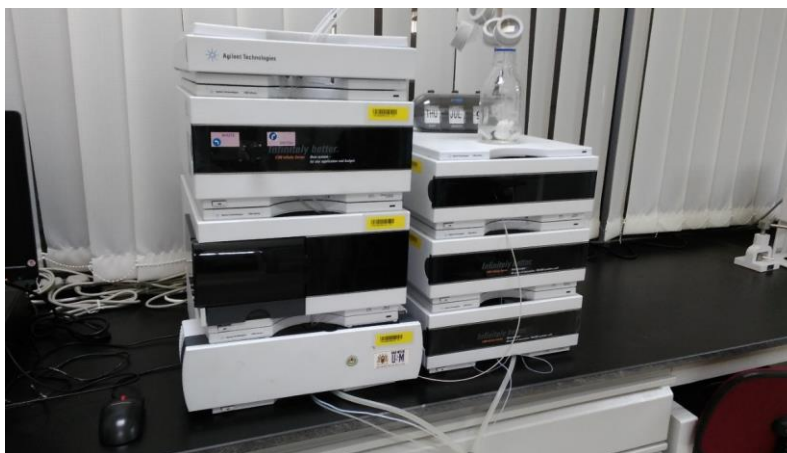
Figure 4. HPLC system used for termiticide analyses
