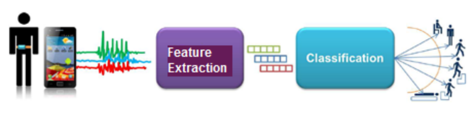
Fig. 1(a). Block Schematic for Activity Recognition Processing
