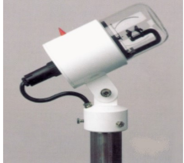
Figure 8 C300R type direct radiometer with sunshine recorder
