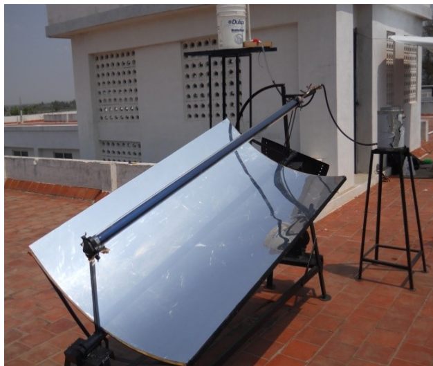
Figure 1 Solar Parabolic Trough Collector System for Cooking
