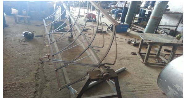
Figure 2 Collector Supporting Structure
