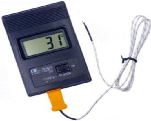
Figure 7 Temperature indicator with K-type thermocouple
