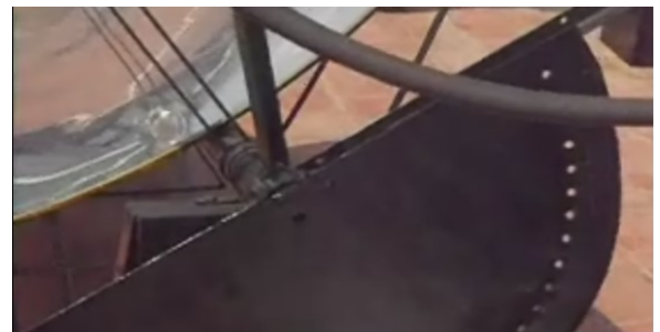
Figure 3 Provisions for Manual Tracking System
